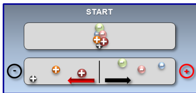
Figure 10. Principle of the electrophoresis
